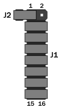
MON08 Connector Jumpered for Standalone Mode Operation
